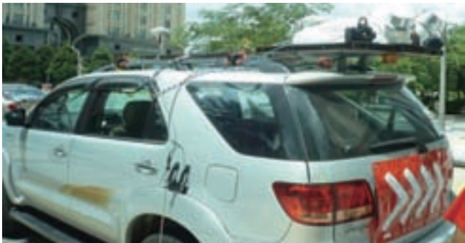
Figure 1. MTLS Dual Laser DynaScan 3 system used
